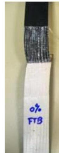
Fig. 3: Unacceptable Weld
