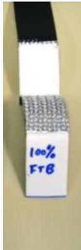
Fig. 1: Acceptable Weld
