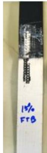
Fig. 2: Partial Weld
