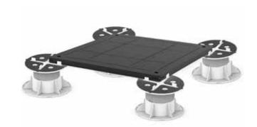
GRO Structural Grates are engineered with a slot cut in each corner enabling a special washer and finishing screw to be inserted. Once all grates are in place, the washer and screw are invisibly screwed into the corresponding screw pad at the top of the pedestal to "lock down" the grates, ensuring a safe, secure, and level surface. Our fastening kit makes removal of a centrally-located grate simple, and eliminates the need to remove all grates from the perimeter up to that point.
