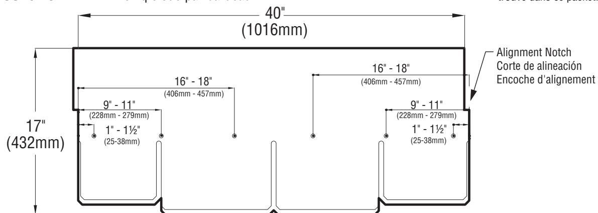
**ENHANCED NAILING PATTERN** - six nails per shingle\*
