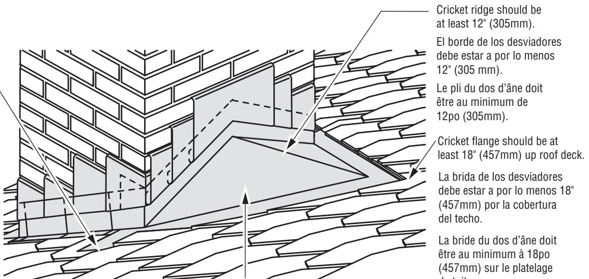
Crickets should extend at least 6" (152mm) up the back of the chimney and extend at least 12" (305mm) up the roof deck.
