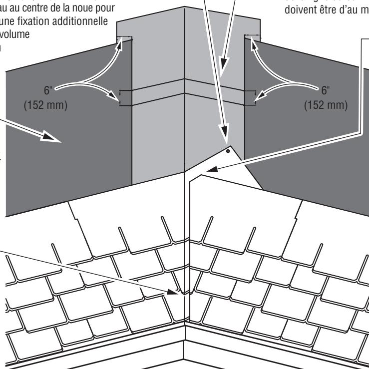
Center full width roll of GAF leak barrier. Do not place fasteners within 6" (152mm) of center line. Horizontal laps must be at least 6" (152mm).
