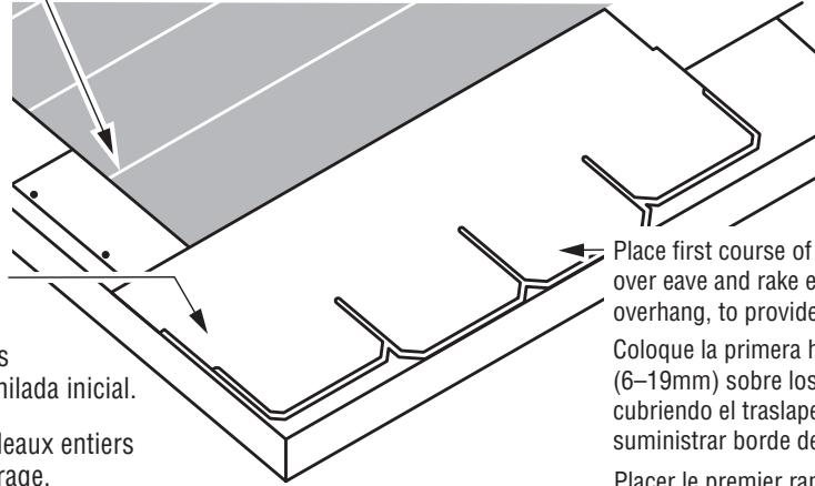
Place first course of shingles 1/4" – 3/4" (6-19mm) over eave and rake edges, covering starter course overhang, to provide drip edge.
