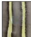
Too Much Part A Slow to rise/no reaction. Yellow in color. Brittle foam after cure.
