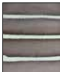
Good Ratio of Part A: Part B Greenish gray in color. Low-rise, tacky foam after cure.
