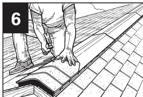
**6** Install new ridge cap in normal manner, using 2-1/2" roofing nails, for 3/4" deck penetration or penetration through the deck, whichever is less. Nailing the ridge caps through the vent along the nailing line will secure the vent. Shingles may need to be trimmed.
