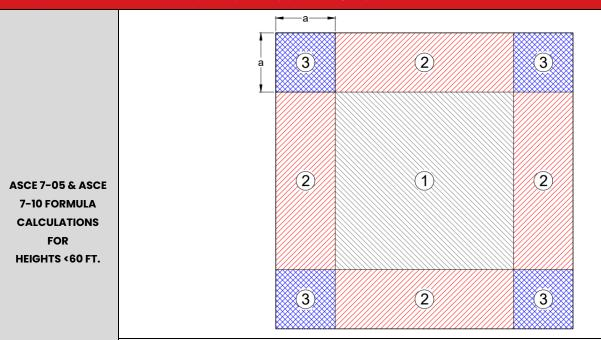
Based on ASCE 7-05 (2009 IBC) and ASCE 7-10 (2012 & 2015 IBC), the perimeter (2) and corner (3) dimensions (a) would be equal to the smaller of the following:
