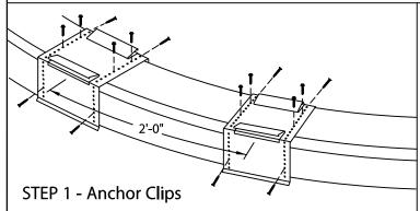
Locate and fasten anchor clips at 2'-0" O.C. with provided fasteners for substrate using the third full hole from bend (see detail A)
