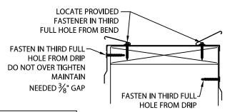
ANCHOR CLIP FASTENING-DETAIL A
