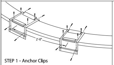
Locate and fasten anchor clips at 2'-0" O.C. with provided fasteners for substrate (see detail A).
