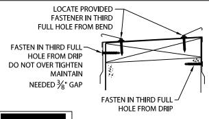
ANCHOR CLIP FASTENING-DETAIL A
