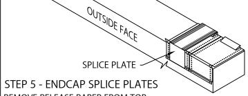
REMOVE RELEASE PAPER FROM TOP OF FACTORY APPLIED SEALANT STRIPS. PLACE SPLICE PLATE ONTO SECOND ANCHOR CLIP AS SHOWN.
