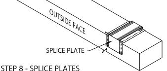
PLACE SPLICE PLATE ONTO ANCHOR CLIPS
