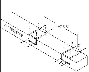
STEP 7 - ANCHOR CLIPS LOCATE OVER MEMBRANE AND FASTEN GALVANIZED ANCHOR CLIPS TO WALL AT 4'-0" CENTER WITH PROVIDED FASTENERS AS SHOWN IN DETAIL A.
