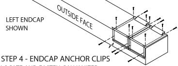
LOCATE AND FASTEN GALVANIZED ANCHOR CLIPS TO WALL WITH PROVIDED FASTENERS FOR SUBSTRATE (SEE DETAIL A).
