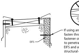
If using an EIFS system, fasten through face w/ fastener of proper length to penetrate through EIFS and attach into structural component
