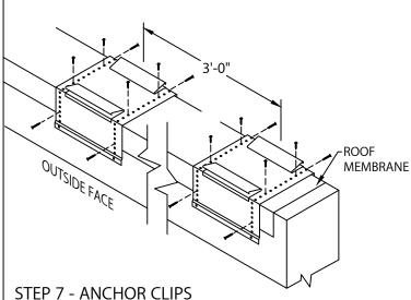
LOCATE OVER ROOFING MEMBRANE AND FASTEN GALVANIZED ANCHOR CLIPS TO WALL AT 3'-0" CENTER WITH PROVIDED FASTENERS AS SHOWN IN DETAIL A
