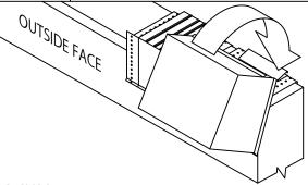
STEP 6 - ENDCAP HOOK OUTSIDE FACE OF ENDCAP OVER THE ANCHOR CLIPS AND ROTATE INTO PLACE.
