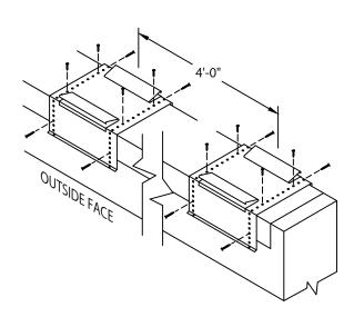
STEP 7 - ANCHOR CLIPS LOCATE AND FASTEN GALVANIZED ANCHOR CLIPS TO WALL AT 4'-0" CENTERS WITH PROVIDED FASTENERS FOR SUBSTRATE (SEE DETAIL A).
