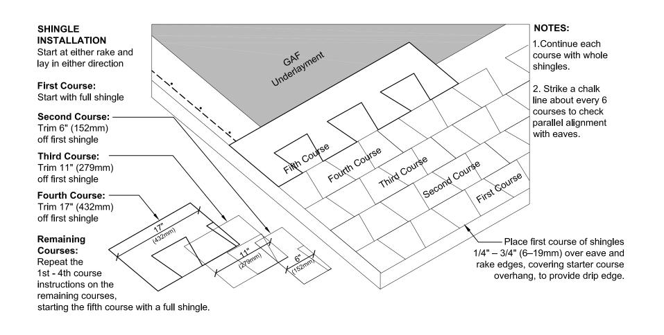
Shingle exposure should be  $5\frac{5}{8}$ " (143 mm).
