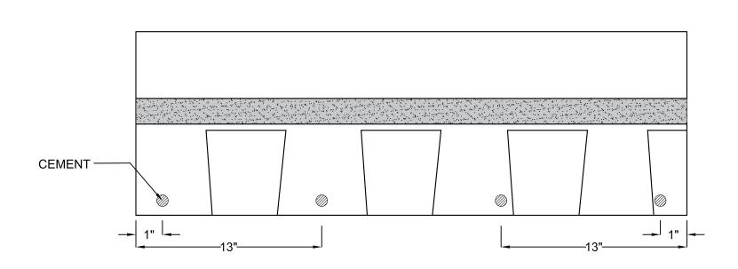
**HAND SEALING**: To hand-seal shingles and to ensure immediate sealing, apply 4 quarter-sized dabs of shingle tab adhesive on the back of the shingle 1" (25 mm) and 13" (330 mm) in from each side and 1" (25 mm) up from bottom of the shingle. Press shingle firmly into the adhesive.
