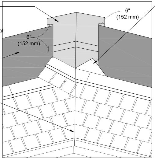
Extend end of shingle at least 12" (305mm) beyond valley center line. Before nailing, firmly press shingles down at valley center to conform to valley shape.
