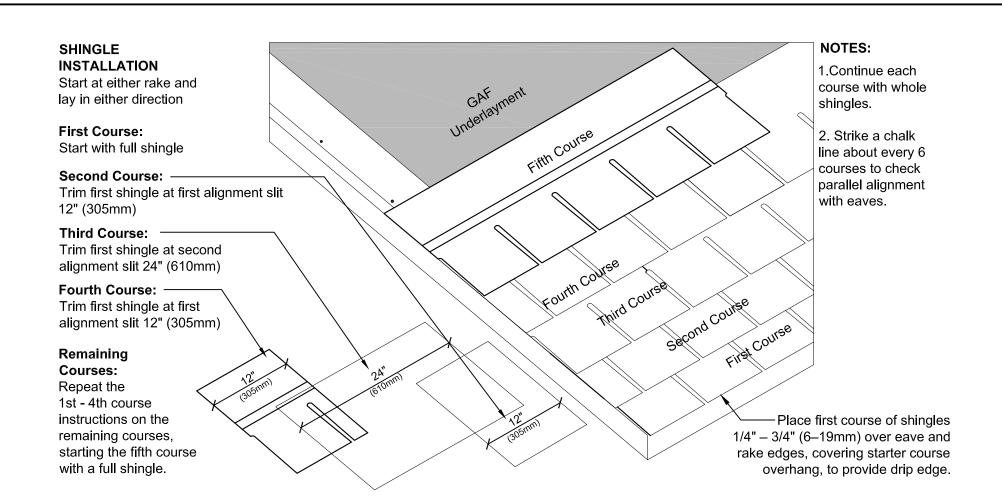
Shingle exposure should be  $7\frac{1}{2}$ " (191 mm).
