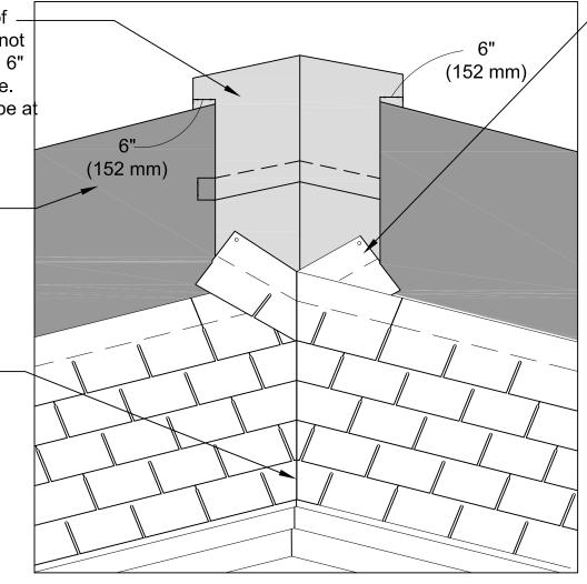
Extend end of shingle at least 12" (305mm) beyond valley center line. Before nailing, firmly press shingles down at valley center to conform to valley shape.
