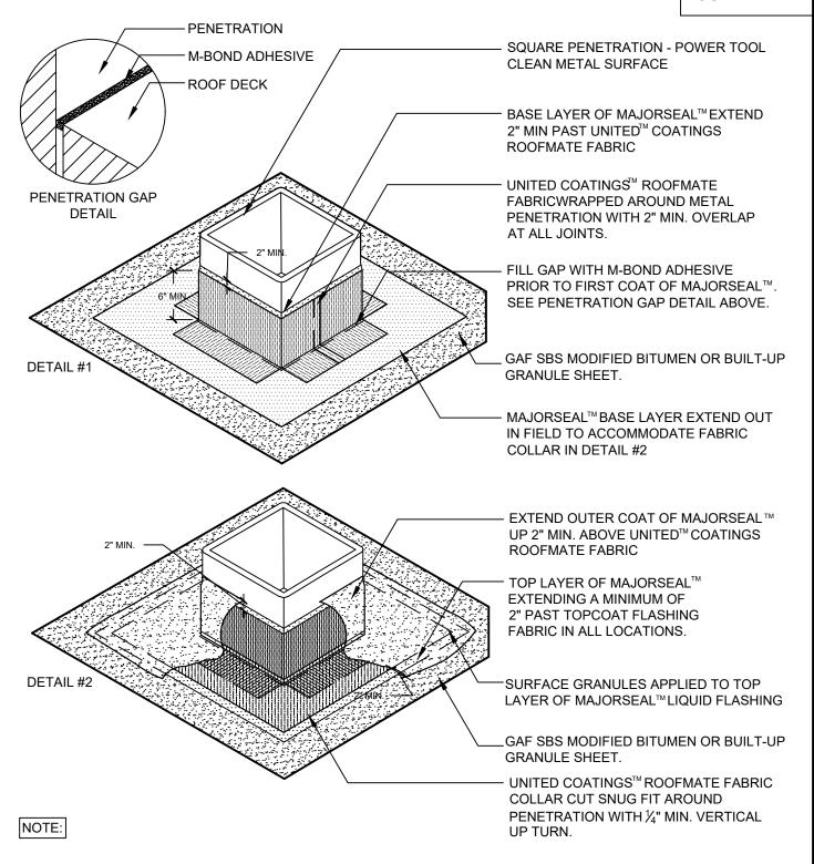
1. PENETRATION GAPS GREATER THAN  $\chi$ " (6MM) REQUIRE BACKER ROD BEFORE APPLICATION OF M-BOND ADHESIVE.
