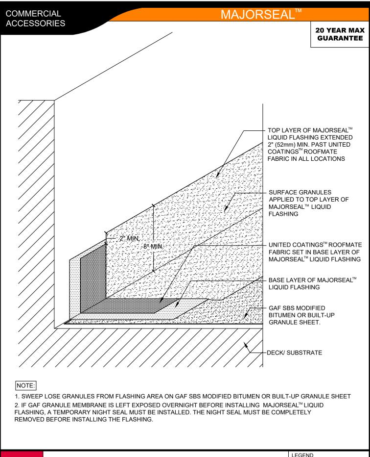
LOW WALL FLASHING DETAIL - 8" MIN.
