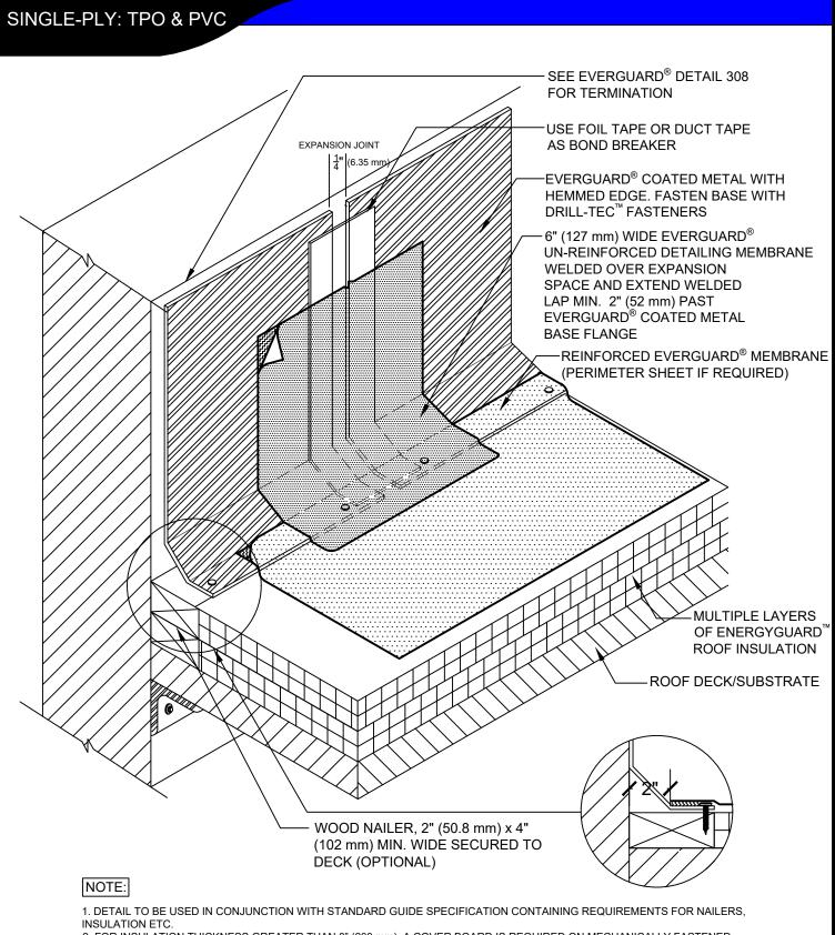
2. FOR INSULATION THICKNESS GREATER THAN 8" (203 mm), A COVER BOARD IS REQUIRED ON MECHANICALLY FASTENED SYSTEMS ONLY.
