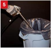
Close valve on cleaner canister and release pressure in hose by squeezing trigger and spraying into a trash bag.
