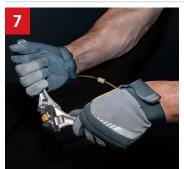
For additional cleaning of the spray tip, if needed, remove it from the extension assembly using a wrench. Hold the flat spots on the extension to keep it from moving. With a second wrench, loosen the retaining cap at the end, carefully remove the spray tip, and soak it in a container with cleaner. Reinstall tip when clean.
