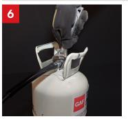
Do NOT disconnect hose unless valve is completely closed. When ready, remove hose and store.
