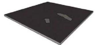
7. **Bleeding / Flushing:** Consistent impact of vehicle tires on asphalt can cause heat and migration of excessive AC to the surface. If surface texture of asphalt becomes filled with liquid AC, it can create a weakened bond for the StreetBond® coatings.
