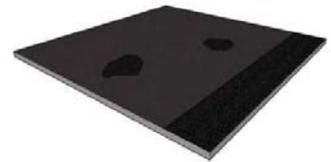
5. **Rutting and Shoving:** Rutting and Shoving is a depression or ripple of the pavement in the wheel path. It is a structural failure due to excessive loading of that pavement. Rutting and shoving is a sign of an unstable asphalt pavement experiencing plastic flow. The pavement's internal structure is not strong enough to bear the weight of vehicle tires.
