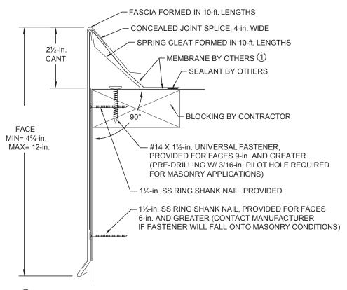
(1) Coordinate installation with membrane manufacturer. (Maximum thickness = 0.060 TPO)
