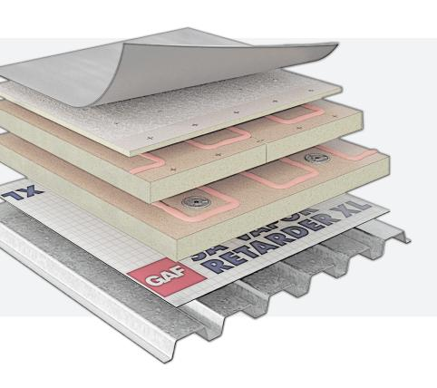
**Deck** — This weight-bearing layer — engineered to support the rest of the roof — may be constructed of thick-gauge steel, wood, or concrete, usually installed atop structural support beams.
