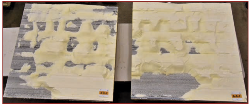
Figure 21. Specimen A-6-2 shown in separated fashion, similar to an opened book. The plane of failure was primarily within the foam core of the top facer of the insulation board (left image), with some delamination at the bottom glass fiber facer of the board (right image).
