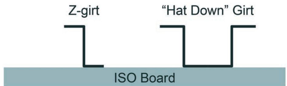
Figure 1. Z-girt and “hat down” girt connect to the sheathing in the same way.
