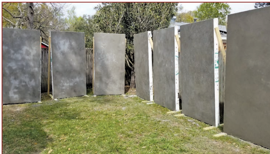
Figure 3. The arrangement of several stucco panels during initial curing.
