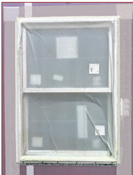
Figure 6. Adhered flashing as installed at window perimeters in test specimens with a building wrap water-resistive barrier (left) and with foam plastic insulating sheathing water-resistive barrier system (right).
