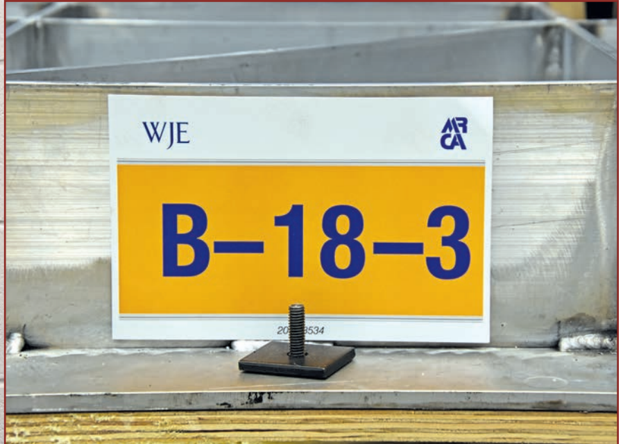
Figure 8. Example of the alphanumeric system and label used to identify the insulation specimens. B-18-3 indicates a cellulosic felt facer (B) with 18 in. ribbon spacing, and specimen number 3.
