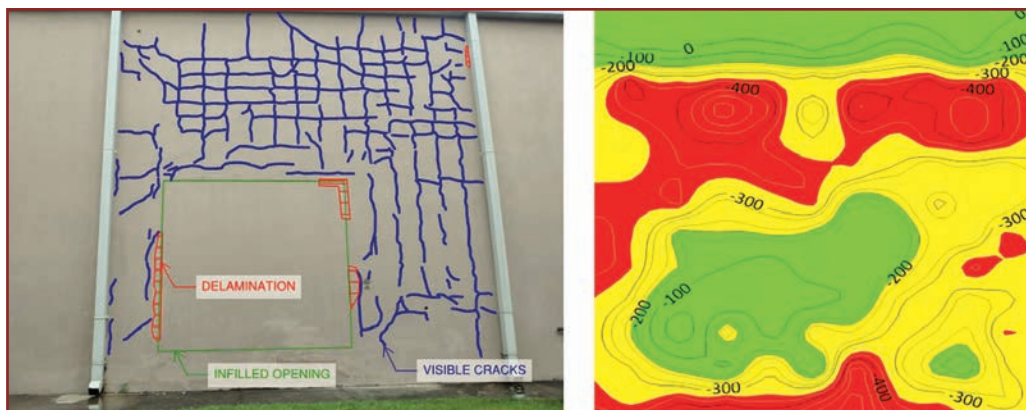
Figure 13. Annotated photograph of wall panel at exterior (left), and half-cell corrosion potential contour map (right). In the map, red and green areas have the greatest and least probabilities for corrosion, respectively, and yellow areas represent corrosion probabilities between those of the red and green areas.
