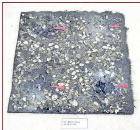
Figure 4. The test sample after the missile drop and after the loose gravel was removed.
