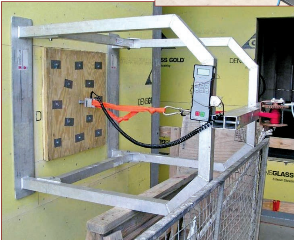
Figure 16. View of an exterior insulation and finish system field pull-test apparatus that is used with test method ASTM E2359. 35 Source: Federal Emergency Management Agency (FEMA P-2062). 4
