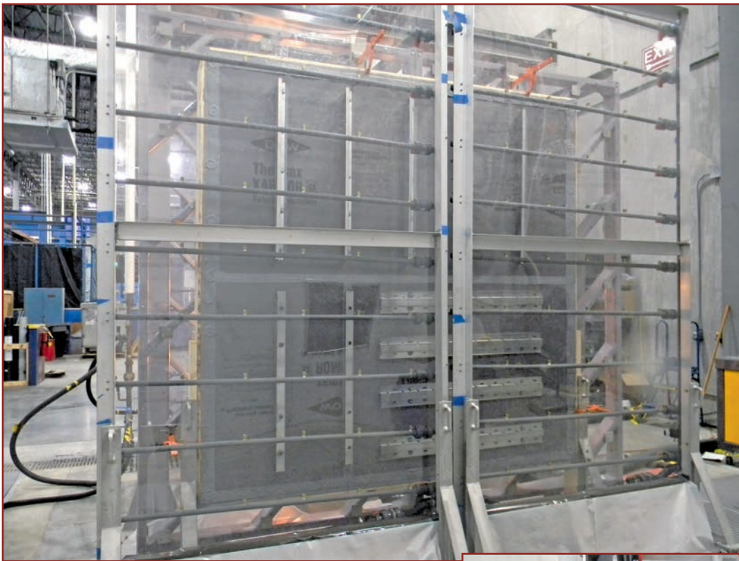
Figure 7. Wall shown in the test setup. Various girts are attached with different flashing configurations. A spray rack is in front of the wall.
