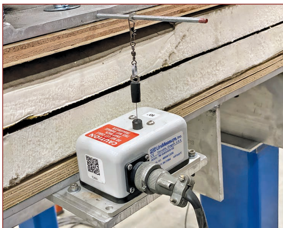
Figure 13. Displacement transducer positioned at the edge of a test specimen to measure separation and elongation of insulation during testing.
