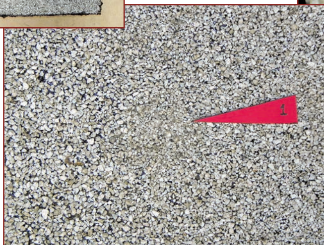
Figure 19. A closer view of impact area 1. There is a slight difference in the color of the granules.
