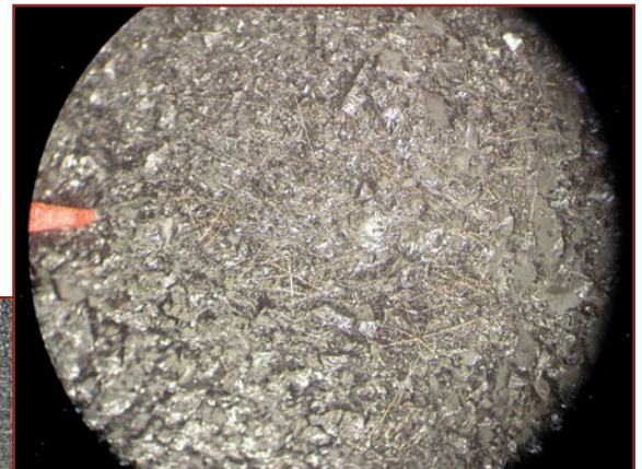
Figure 12. Impact area 4 at 10-power and the crushed interply asphalt at the point of impact.
