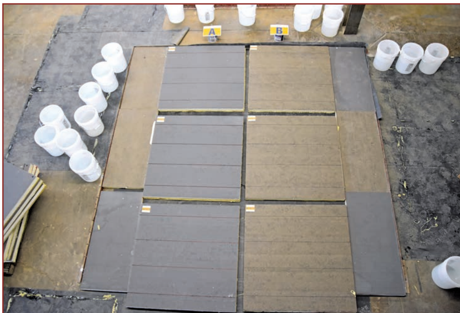
Figure 1. Lines were drawn on the insulation boards (with spacings centered on boards) to guide the application of the low-rise foam adhesive ribbons. The lines were centered so that application of the adhesive would be symmetrical. The photo shows the line layout for a 12 in. ribbon spacing.
