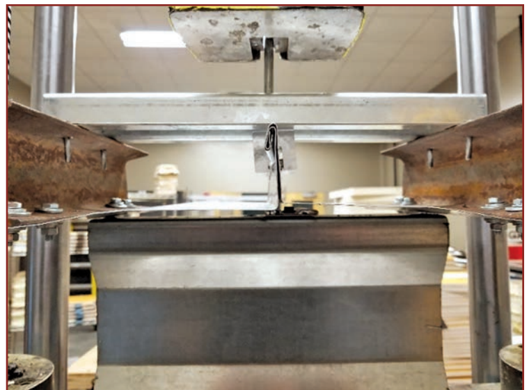
Figure 7. Small-scale test to estimate enhanced strength of a standing seam roof with external seam clamps.
