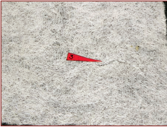
Figure 16. Magnified view of the fracture in the felt at impact area 3.
