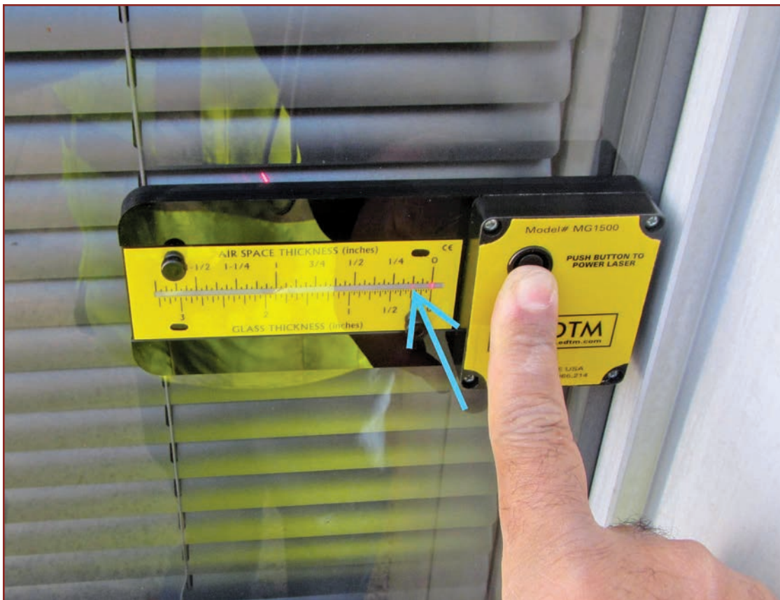
Figure 11. Glazing thickness measurement (1/2 in.) at curtainwall glazing panels.
