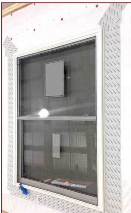
Figure 6. Adhered flashing as installed at window perimeters in test specimens with a building wrap water-resistive barrier (left) and with foam plastic insulating sheathing water-resistive barrier system (right).
