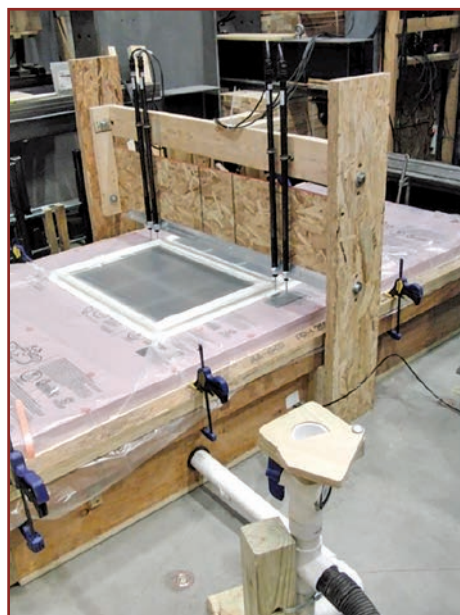
Figure 7. ASTM E330 23 test apparatuses used to evaluate uniform pressure resistance. Figure: Qualtim/Center for Building Innovation (left); Home Innovation Research Labs (right).
