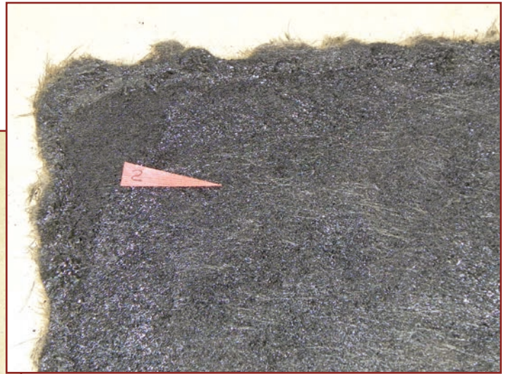
Figure 9. Close-up of impact 2 with no evidence of crushed or disturbed interply.
