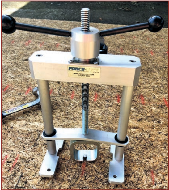
Figure 1. View of a fastener being extracted from an oriented strand board panel with a digital pull tester.
