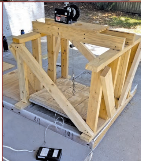
Figure 5. The overall arrangement of the stucco pull-test rig. A worm-gear-driven winch was used to apply tension to a cable connected to an eyebolt in the plywood blank. A 1000-lb load cell was placed in line between the tension cable and the eyebolt.
