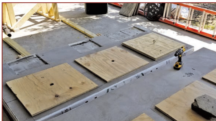
Figure 4. Stucco panels being prepared for testing. The panels were removed from the support stands and laid flat. Per ASTM C1860, nine 3/4-in.-thick plywood panels were adhesively attached to the stucco.
