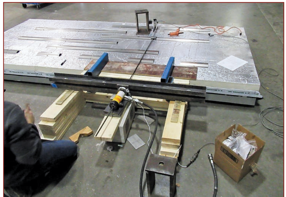
Figure 14. Testing apparatus developed by the authors to quantify key performance features of surface-mounted connections on a structure with a relatively heavy veneer.
