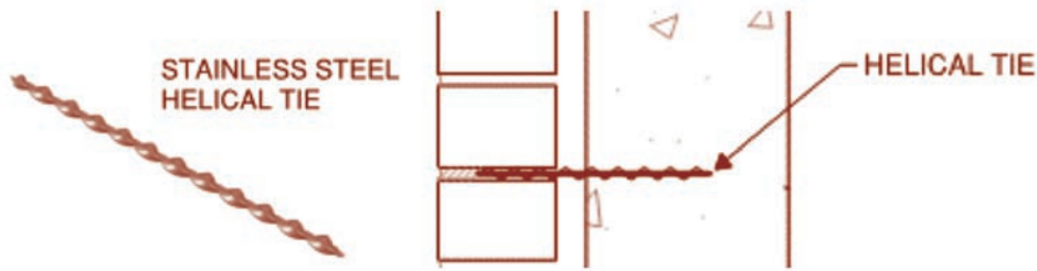
Figure 2. General detail for helical ties for a brick veneer system.
