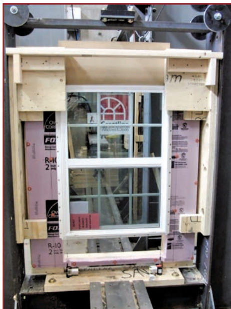
Figure 9. Window installation shear load test setup.
