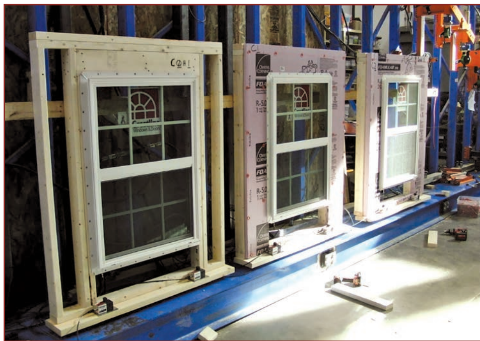
Figure 8. Sustained dead load tests for creep and stability. Figure: Qualtim Inc. 2013. Creep of Fasteners Installed into Windows over Foam Sheathing Panels and OSB. Madison, WI: Qualtim Inc.
