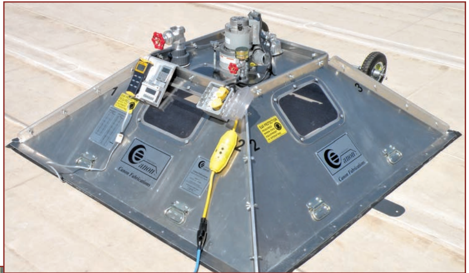
Figure 15. View of a negative pressure test apparatus that is used with test methods ASTM E907 33 and FM Global Property Loss Prevention Data Sheet 1-52. 34
