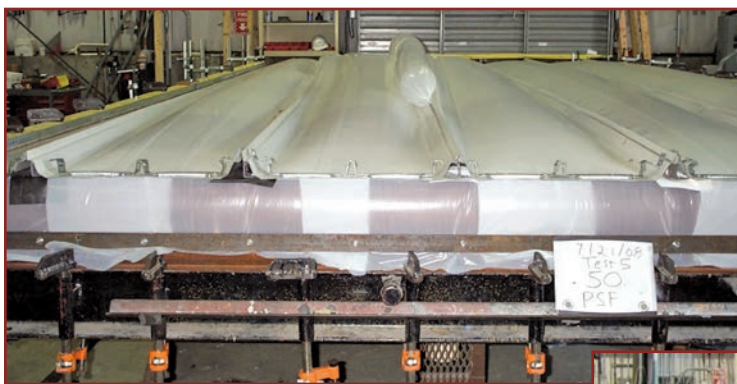
Figure 5. Large-scale testing of a standing seam roof (SSR) without external seam clamps (ESCs) (above) and with ESCs that did not fit the SSR properly (at right). Compared with the failure point for the SSR with no ESCs (50 lb/ft 2 ), the failure point for the SSR with improperly fitting ESCs only increased by 20% (to 60 lb/ft 2 ).
