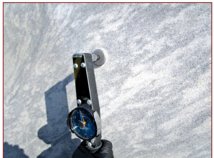
Figure 10. Installed custom stone anchor into the marble cladding (left) and torque testing (right).
