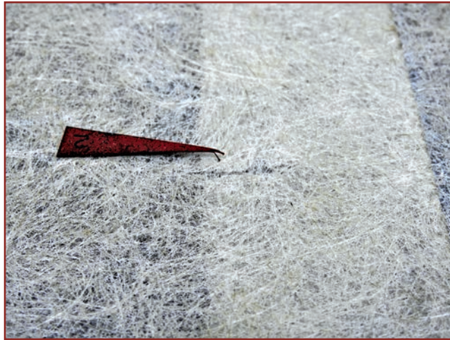
Figure 41. Fractured bottom ply of the membrane.
