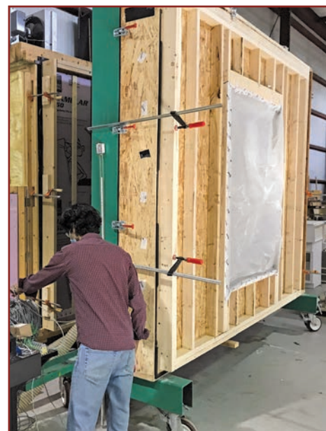
Figure 7. ASTM E330 23 test apparatuses used to evaluate uniform pressure resistance. Figure: Qualtim/Center for Building Innovation (left); Home Innovation Research Labs (right).
