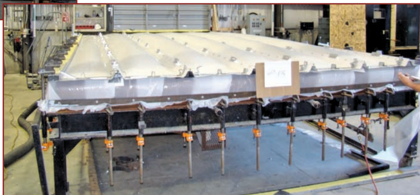
Figure 5. Large-scale testing of a standing seam roof (SSR) without external seam clamps (ESCs) (above) and with ESCs that did not fit the SSR properly (at right). Compared with the failure point for the SSR with no ESCs (50 lb/ft 2 ), the failure point for the SSR with improperly fitting ESCs only increased by 20% (to 60 lb/ft 2 ).
