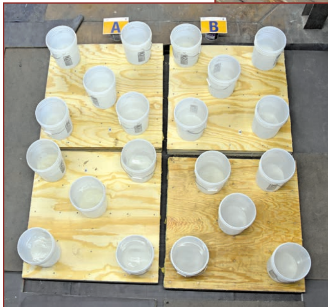
Figure 4. Typical weights used as ballast until the foam adhesive set up, typically for 10 to 15 minutes per specimen.
