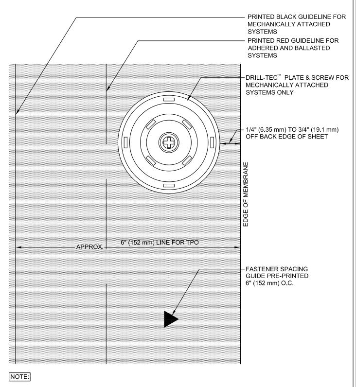
1. APPLY EVERGUARD® TPO CUT EDGE SEALANT TO ALL CUT REINFORCED TPO EDGES (REFER TO EVERGUARD® DETAIL 115).
