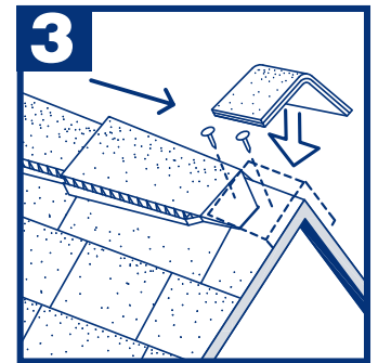
Cover... the tabs of the last Vented RidgeCrest™ piece with two layers of shingle fabric or a trimmed piece of Vented RidgeCrest™.
