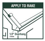
**RAKE APPLICATION:** After installing the drip edge, set and nail Elk Starter Roll into place the full length of the rake, starting at the lowest edge of the rake. Overhang the rake approx. 1/2" (1.3 cm) to obtain a straight edge reveal for rake edge shingle application. Make sure WindGuard sealant is facing up and nearest the outermost edge of the rake.
