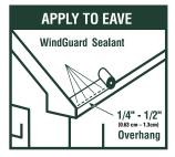
**EAVE APPLICATION:** After installing the drip edge, set and nail Elk Starter into place the full length of the eave edge. Overhang the starter roll 1/4" (0.63 cm) – 1/2" (1.3 cm) to obtain a straight drip edge. Make sure WindGuard sealant is facing up and nearest the lowest edge of the eave.
