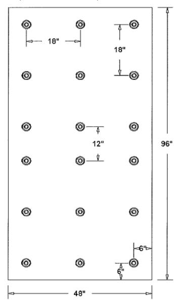
**Note 3:** 16 Fasteners per 48"x96" board attachment pattern:
